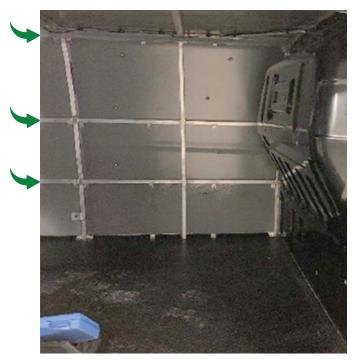
The Modul-Rail are glued to the three thin horisontal beams of the vehicle
