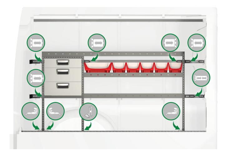
UV-bracket fixed between partition wall and racking to stop inwards rotation.
