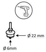
Position the template in the vehicle, remove the center drill and drill carefully down to the honeycomb.
